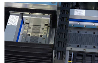
Linear actuators of X- and Y-axis
